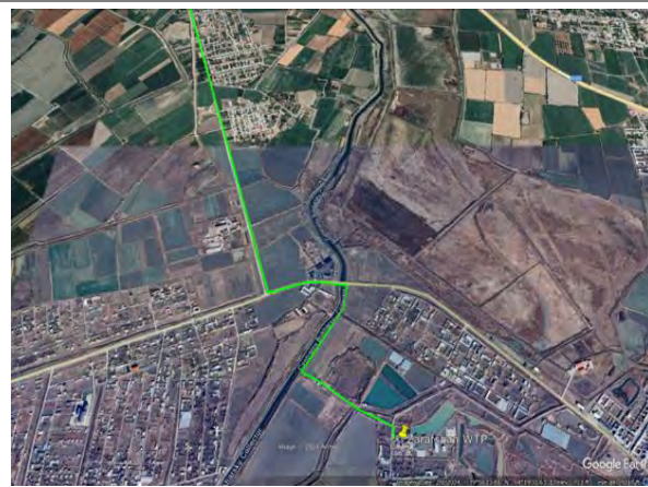
(b) Water main (green line) starting in Zarafshan WTP and running along the Central Bukhara Drainage Canal
